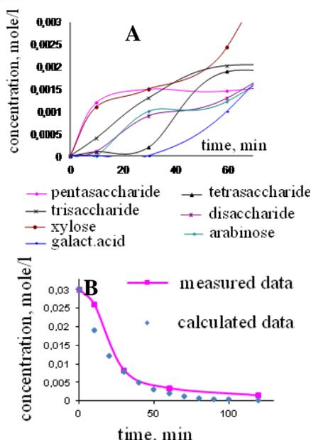
Figure 3: Catalyst composition after xylan hydrolysis with the enzyme complex (pH 4.8,  $t=40^{\circ}\text{C}$ ,  $m_{\text{enzym prep}}=0.42\text{ g}$ ,  $V_{\text{react.mix}}=15\text{ ml}$ ): a) accumulation of hydrolysis products, b) initial polysaccharide substrate conversion.
