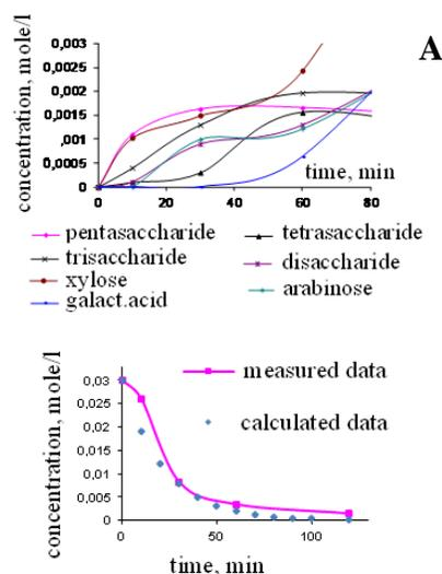
Figure 4: Catalyst composition after xylan hydrolysis with the catalyst (pH 4.8,  $t=40^{\circ}\text{C}$ ,  $C_{\text{cat}}=0.6\text{ g}$ ,  $V_{\text{react.mix}}=15\text{ ml}$ ): a) accumulation of hydrolysis products, b) initial polysaccharide conversion.
