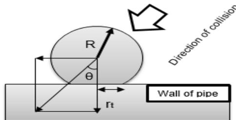
Figure 2 - Particle collision and deformation
