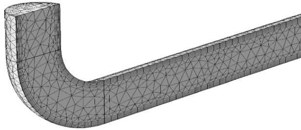
**Figure 3** - Meshing scheme of the tube
