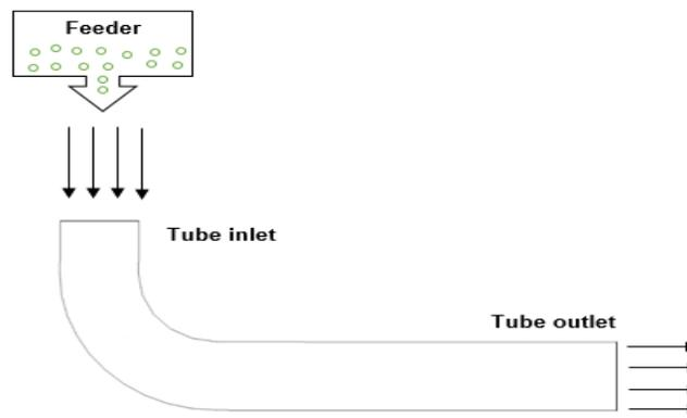
**Figure 1:** The schematic of the conveying process to be simulated
