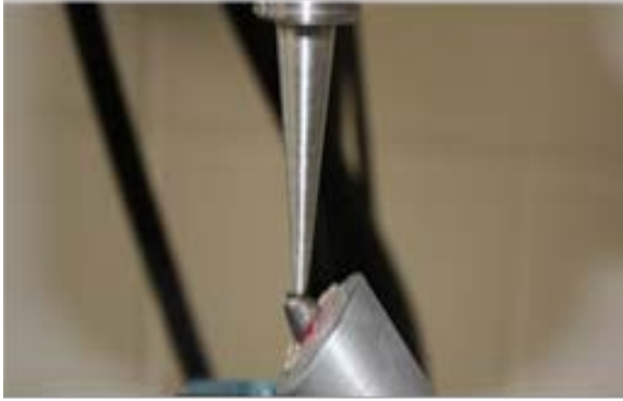
Figure 1: Image showing test specimen orientation in Instron mashine.
