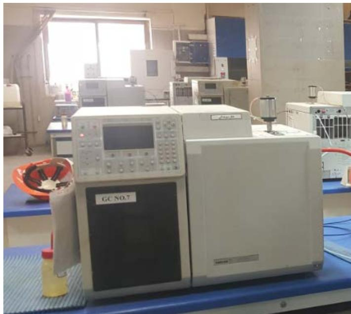
**Fig. 4:** AmirKabir petrochemical GC device (CP-SIL5CB, Varian 3800)
