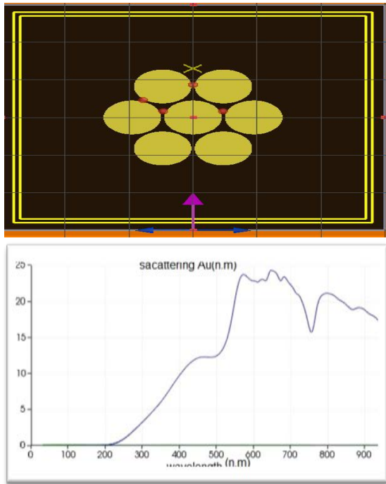
Fig. 6: shows the heptamer scattering spectra occurs with carbon dielectric nano-particles that has a fano-resonance at 737 nm. As a result, adding nanoparticles to the metal cluster increases the coupling between nano-particles without reducing the physical distance between nanoparticles. Four polar modes are observed at 450 nm.
