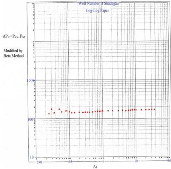
**Figure 5:** Log. Curve of data of Shadgan well number B after the elimination of wellbore storage effect by Beta method
