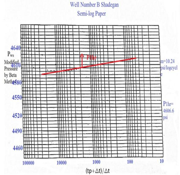
**Figure 6:** semi-log. Curve of data of Shadgan well number B after the elimination of wellbore storage effect by Beta method
