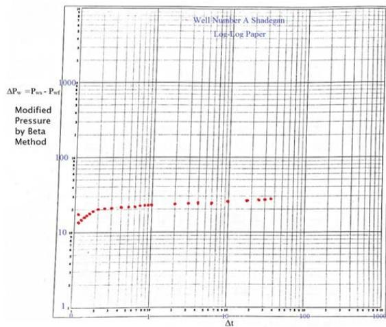
Figure 3: log. Curve of Shadgan well number A after the elimination of wellbore storage effect by beta method
