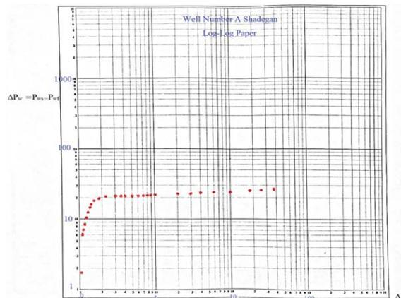
Figure 1: log. curve of build-up pressure test of Shadgan well number A
