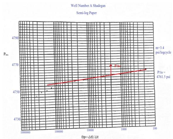
Figure 2: semi-log curve of build-up pressure test of Shadgan well number A
