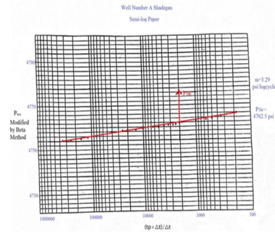
Figure 4: semi-log. Curve of Shadgan well number A after the elimination of wellbore storage effect by beta method
