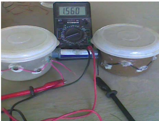
Fig. 1 Experimental set-up for single dual chambered MFC.
