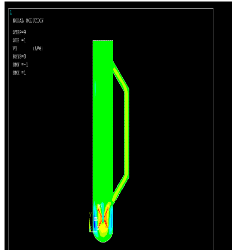
Fig. 6: Flow patterns of the fluid at an air velocity of 1 m/s (cross-shaped sparger).
