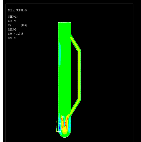
Fig. 10: Flow patterns of the fluid at air velocity of 3.0 m/s (cross-shaped sparger)
