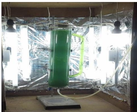
Figure 11: Culturing Anabaena ambigua in an external loop airlift photobioreactor at a light intensity of 80 \mu\text{mol}/\text{m}^2\text{s} .
