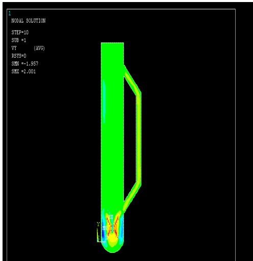
Fig. 8: Flow patterns of the fluid at an air velocity of 2 m/s (cross-shaped sparger).
