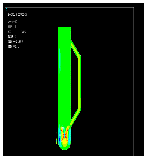
Fig. 9: Flow patterns of the fluid at an air velocity of 2.5 m/s (cross-shaped sparger).
