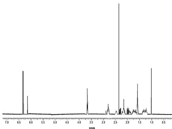
**Figure 5.** The scheme showing the  $^1\text{H}$ NMR spectrum from compound **7** analyzed with a Varian VXR300/5 FT NMR apparatus at 300 MHz in  $\text{CDCl}_3$ . Axis abscissa (ppm). ppm = parts per million.
