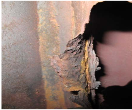
Figure 2: Tube damage at higher resolution
