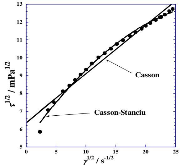
**Figure 6.** Variation of the square root of shear stress of ketchup with the square root of shear rate at different temperatures. Dots (●) represent experimental values and lines represent linear and non-linear fits.
