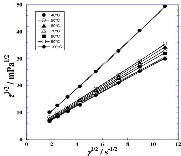
**Figure 1.** Variation of the square root of shear stress with the square root of shear rate at different temperatures. Dots represent experimental values and lines represent linear and non-linear fits.
