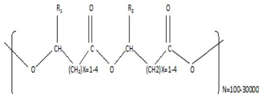
**Figure 2.** Structure of Polyhydroxyalkanoates with  $R_1$  and  $R_2$  are alkyl groups (C-C)
