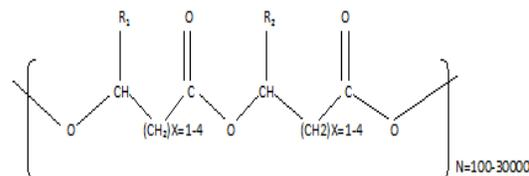
**Figure 1.** Structure of Polyhydroxyalkanoates with R<sub>1</sub> and R<sub>2</sub> are alkyl groups (C-C)
