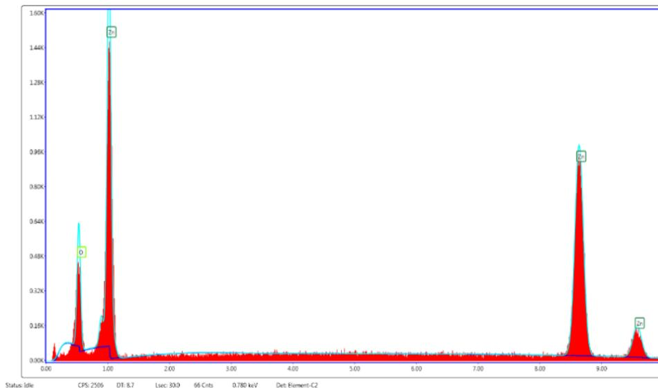
**Figure 1.** Energy Dispersive X-ray (EDX) spectrum of synthesized ZnO nanoparticles. The spectrum confirms the elemental composition with prominent peaks corresponding to zinc (Zn) and oxygen (O), validating the formation of ZnO nanoparticles.
