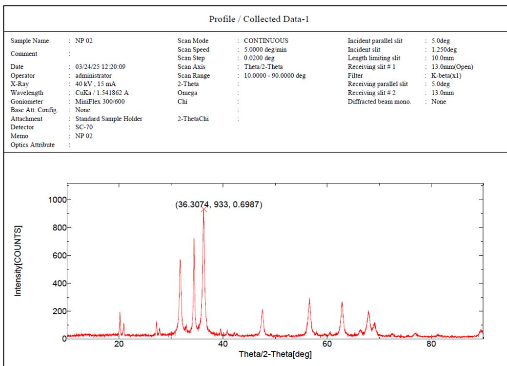
**Figure 4.** XRD pattern of ZnO nanoparticles synthesized using *T. cordifolia* extract, showing distinct peaks corresponding to the hexagonal wurtzite structure.
