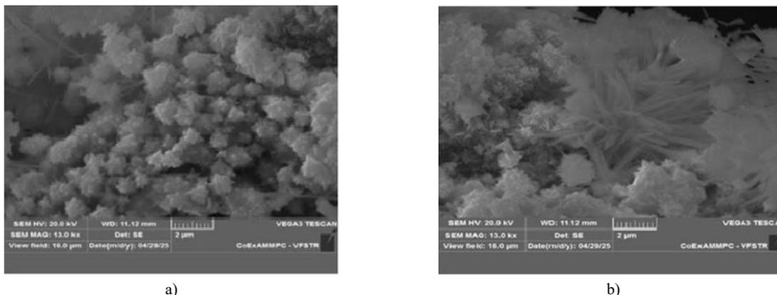
**Figure 2.** SEM micrographs of green synthesized zinc oxide particles using *T. cordifolia* extract. a) Densely aggregated, quasi-spherical particles with rough surface morphology, b) Mixture of spherical aggregates and needle-like or rod-shaped nanostructures
