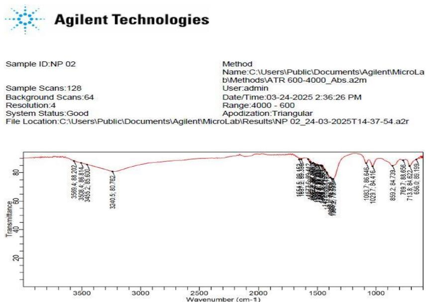
**Figure 3.** FTIR spectrum of ZnO nanoparticles synthesized using *T. cordifolia* extract, showing characteristic Zn–O stretching vibrations and functional groups from plant phytochemicals.
